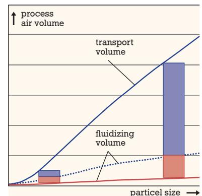
**Region of operation for fluidized bed (blue) and extended region of operation for ProCell (red)**
